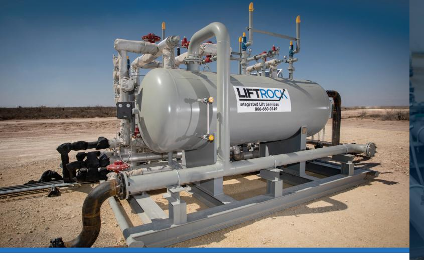
QuickSet<sup>™</sup> by Liftrock<sup>™</sup> is the revolutionary gas lift control system that delivers unmatched environmental and economic advantages. The patented, scalable, skid-mounted QuickSet system eliminates fugitive methane emissions, while also significantly cutting construction time and costs. In addition, this advanced system also eliminates the need for liquid-dump methanol line injections and scrubber dump events.
