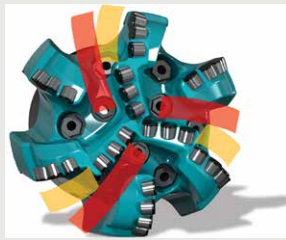
Figure 2. SplitBlade features separation of the primary blades, creating double barrel hydraulics that free up more area for the junk slot.
