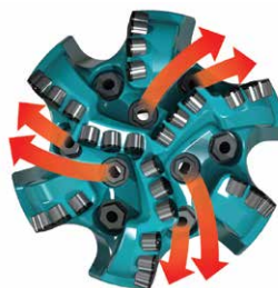
Fig. 3. The new PDC design features separation of the primary blades, creating double-barrel hydraulics that free up more area for the junk slot.
